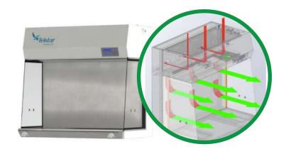
Telstar Aeolus H horizontal laminar flow hoods provide a protected space and allow for sterile, particle-free working conditions. *The product can be handled without risk of contamination by the environment or the operator.*
